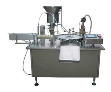
This machine is suitable for filling and sealing to easy-folding plastic bottle.
