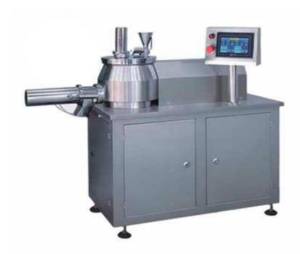
HLSG-30 High shear mixer granulator is a new generation of granulating equipment developed by our company, which can finish the procedures of mixing, wetting, granulating in one time. Which is very effective and in compliance with GMP standard.
