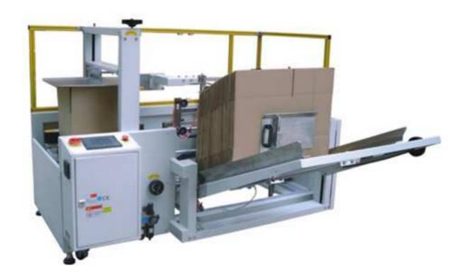
The working process of the carton erector is open the carton, carton in shaped, bend the carton bottom and seal the bottom with adhesive tapes. After the carton bottom is bend and sealed, it will convey to the carton packing machine. The carton erector is widely used in the automatic carton packing industry. The whole process is controlled by the PLC and touch screen. It is a necessary part in the automatic packing process.
