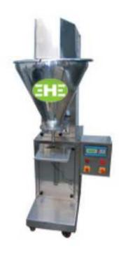
Semi Powder Filling Machine is used to fill variety of product like granules, powder etc in bottle and Pouch. It basically works on Auger base to fill powder in bottle and Pouch.
