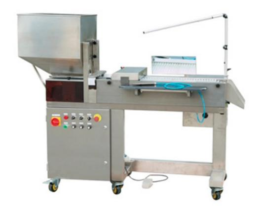
HB-220 model drug inspecting machine is a new product researched by our company on the basis of integration of domestic and foreign advanced technologies in order to meet the needs of pharmaceutical sector. It can test outlook quality for hard capsules, soft capsules caplets and tablets.
