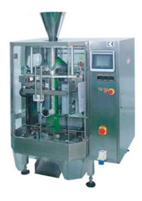
Has been designed to meet the demand of large rates. Flexibility, ease of maintenance, ease of settings, synchronization with the power systems, flexibility, and quiet operation have been our priorities in the design of this machine. It provides an output up to 10-40 bags/minute.
