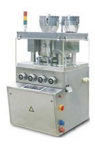
ZPS37A rotary tablet press is a new generation product which is developed form the former ZP37 Tablet Press and it's a continuously automatic rotary tablet press for pressing tablets, it is widely applicable to industries such as pharmaceutical, chemical, foodstuff and electron for pressing the granular materials into all kinds of round tablets, irregular tablets, two colors tablets and ring shaped tablets.
