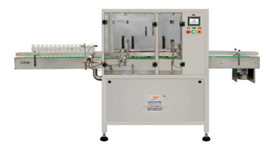
The Automatic Linear Air Jet Vacuum Cleaning Machine consists of the main structure, product infeed screw, in-feed star plate, pneumatic component, washing nozzles, electrical panel, AC drive & motor.
