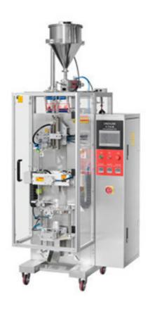
DC-890A fully automatic single/double-row back-seal packaging, suitable for back-seal strip packaging of liquid, powder, granular, and other materials in the food, pharmaceutical, and daily chemical industries.
