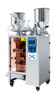
Applicable to the automatic packaging of liquid paste products in the cosmetics industry, such as: a black wash + double oxygen milk, shampoo + conditioner, shampoo + shower gel, etc.; divided into left and right compartments and front and back compartments, while measuring 2 Different materials.
