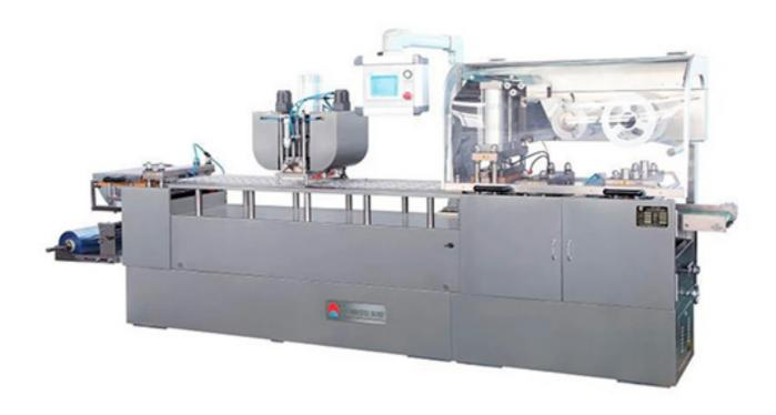
This Chocolate Blister Packing Machine was innovatively developed by our own company. It is suitable for packaging chocolates, butter, biscuits, perfume, essence, facemasks etc with AL/PL, PL/PL materials. It is equipped with a micro-computer control system and frequency converter, with characterized by higher automation and easy operation. It is popular equipment for the foodstuff and cosmetics, particularly for those who are to make their own career.
