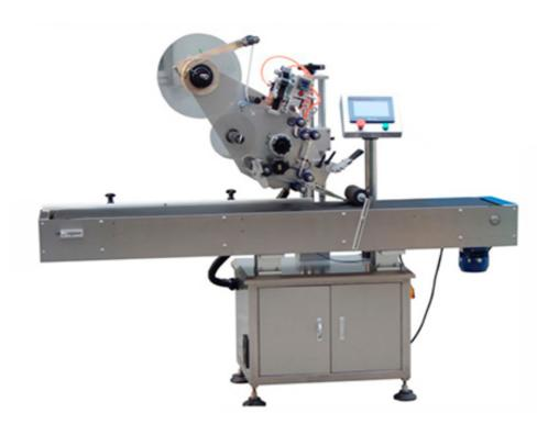
Applicable to the pharmaceutical, cosmetic, food and packing and so on a variety of industries in rigid package or soft packing material of flat surface and uneven surface automatic labeling.
