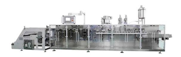
BHD-240S is specially designed for standard stand-up pouches with larger size and higher loading capacity. The loading capacity can be up to 2000ml. It is commonly used to package soy milk, candy, laundry detergent, peanuts, nuts, cashews, etc. It can also be packaged according to customer needs. Design hooks, special shapes, zippers, suction nozzles and other functions.
