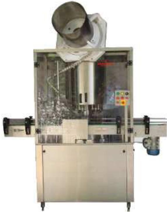
On-line filled containers are fed and guided on the moving SS/Plastic slat conveyor belt at the required speed of the correct placement below Capping Head. The filled bottle moving in star wheel pick up cap from the cap chute and move under the Capping head for perfect ROPP Capping.
