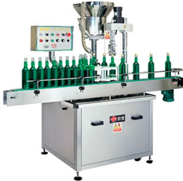
The container cap closing processor is capable to be applied for both plastic screw caps and ROPP sealing caps in one machine by changing capping system components. Capping system is designed with mechanical torque limit device to prevent over capping which damages the cap appearance.
