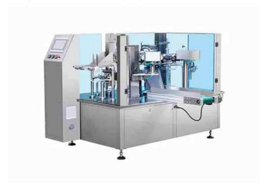
Fully automatic completion of all production processes such as feeding, automatic bag pickup, coding, bag opening, quantitative filling, heat sealing and finished product output.
