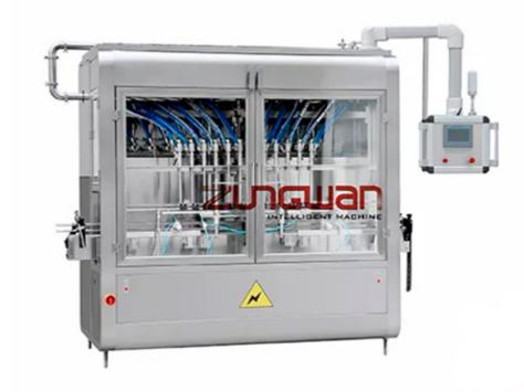
This liquid filling machine is our newly developed filling machine. It has reached the international advanced level, partial has exceeded the similar product. It is abroad, also certified by the world famous chemical magnate. This is a inline piston filling machine for cream and liquid
