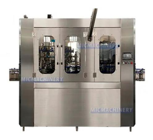
MIC 18-6 beer canning equipment adopts isobaric pressure filling system which is applicable for beer (Cold filling temperature at 0-4 degrees Celsius)
