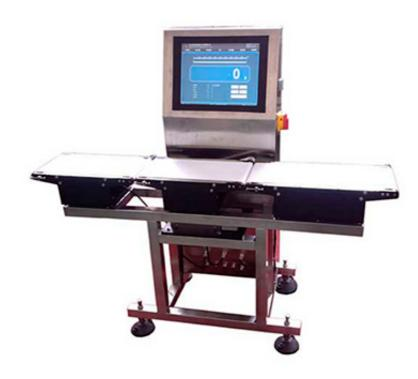
The checkweigher machine detects the weight of the known objects. When the weight of the object exceeds the allowable upper and lower limits, the checkweigher system will automatically detect the out-of-tolerance, and can automatically remove it from the production process and give an alarm signal.
