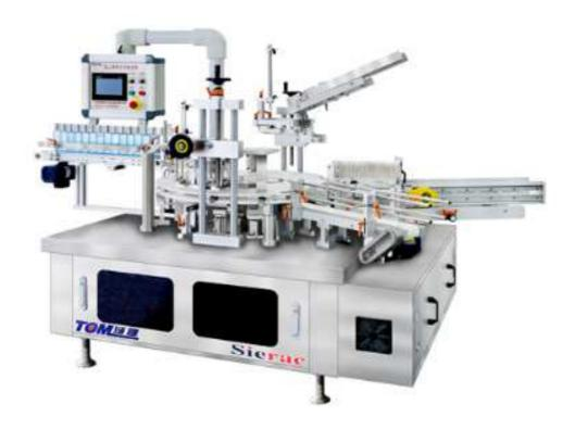
The new series cartoning machine built with "BALCONY" design, allowing the mechanical working parts separated from the packaging area. It respects the present accident prevention maintenance and hygienic laws. The machine works with intermittent motion and with electric synchronisms controls, PLC and touch display control system functions recall-able; it is possible memorizing 100 menus with relative data for 100 different productions.
