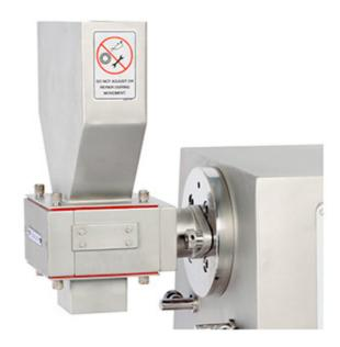
An ideal to granulate tablets, slugs and pellets. The Dry Granulator – SDG consists of two motor-driven rollers with teeth force. This forces the material to be granulated with a very low proportion of powder. Hard slugs of 2 to 2.5 mm thick the following granulation will be obtained, 50% of 16 mesh, 25% of 24 mesh, 10% of 70 mesh and 20% of the powder.
