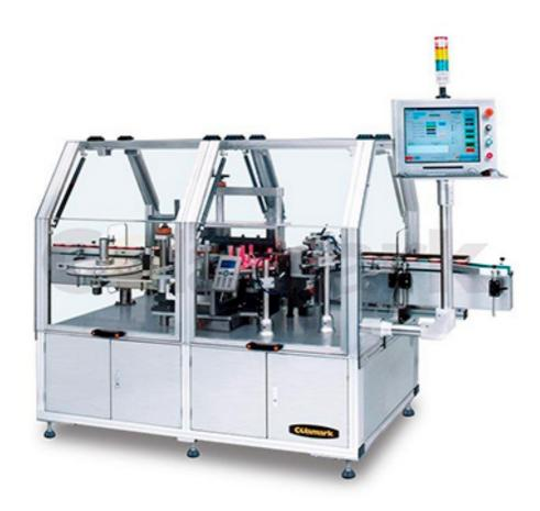
With all the functions of the A117, the A117R is specially designed to also fulfill the demanding requirement that when putting two labels on one bottle, the labels have to be symmetrically aligned on the bottle irrespective of the bottle diameter variation.
