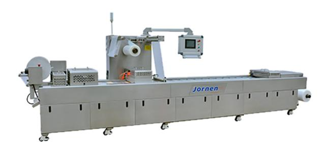
These DFP series of Thermoformer has been designed to pack food and medical products, capable of both flexible and rigid packaging.
