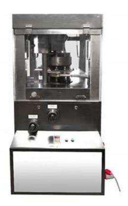
This Granulator Machine is suitable for food, medicine, chemical, electronics and other industries to press granular raw materials into circular sheet/block/ball/ring sheet, shaped sheet and other shapes. Not suitable for solid, wet particles, low solubility, hygroscopic raw materials and no particles and fine powder materials pressing. The machine meets the GMP standard requirements.
