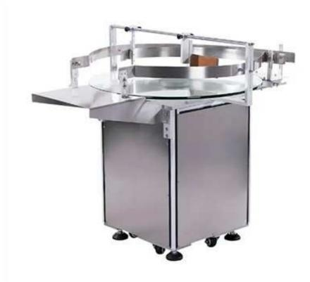
FKA-601 Automatic Bottle Unscramble machine is used as a supporting equipment to arrange the bottles during the process of rotating the chassis, so that the bottles flow into the labeling machine or the conveyor belt of other equipment in an orderly manner according to a certain track.
