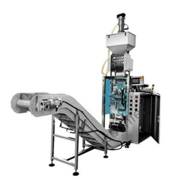
High speed liquid multi lanes packing machine is suitable for packing different kinds of liquid. Such as: honey stick, jelly stick, sauce sachet, oil sachet etc.
