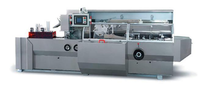
YL-300P High speed cartoning machine can fold leaflet, open box, insert blister into box, emboss batch number and close box automatically. The highest speed can up to 260 boxes/min.
