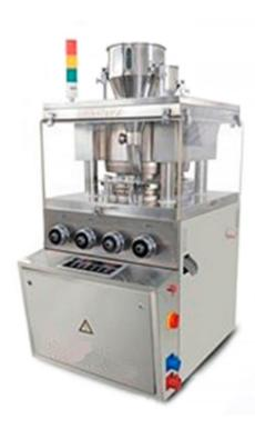
The machine is a new generation product which is developed form the former ZP series Tablet Press of my company, it is a double-press type, continuously automatic rotary tablet press for pressing tablets, it is widely applicable to industries such as pharmaceutical, chemical, foodstuff and electron for pressing the granular materials into all kinds of round tablets, irregular tablets and ring shaped tablets.
