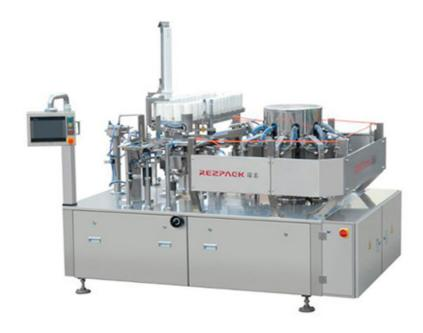
Vacuum Chamber machines or Vacuum packing machines are used to evacuate the air around perishable goods such as food products like meet, beef, chicken wing, drumstick, corn and other block-type materials whose extension of shelf life is desired.
