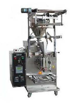
Automatic powder packaging machine is new-updated compact version pouch pick fill seal packing machine for various pre-made bags such as pillow bags, gusset bags, zipper bags etc. As a cost saving solution, it is ideal for a lot of application such as all kinds of powder material like: Tea powder, wheat flour, coffee powder, coco powder etc.
