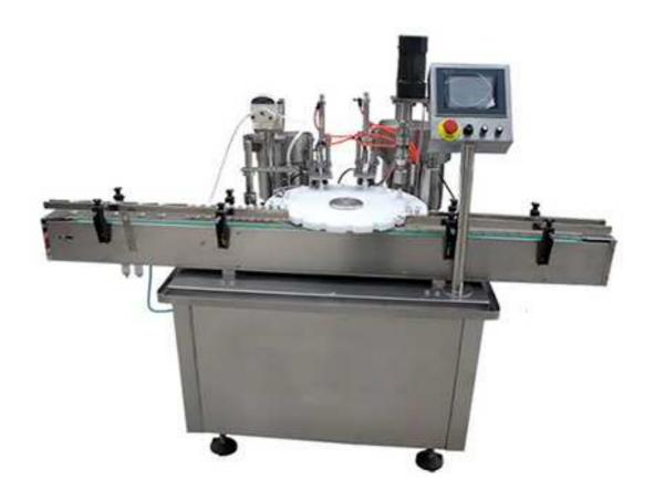
This machine is filling and capping equipment for dropper bottle, advanced design, reasonable structure, can automatically complete filling, sorting and capping process. no bottle no filling, and other functions. Can be used stand-alone, and also can be used for filling line. This machine completely accords with GMP requirements.
