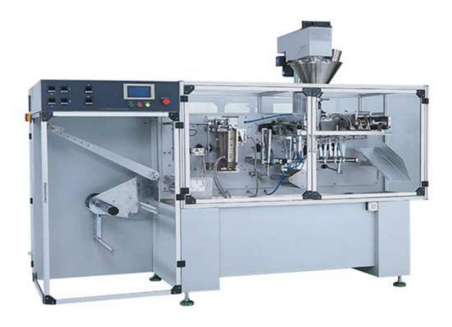
This machine uses PLC control, with precise bag-making dimensions and high metering accuracy. The machine runs smoothly and is more suitable for 24-hour continuous operation. The filling method is flexible, with options such as screw, cup, seagull, and piston, suitable for various materials. It can achieve various international standard sealing methods.
