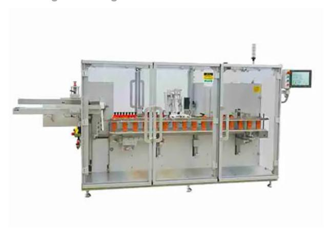
The main difference between the ring intermittent vertical cartoning machine and the horizontal cartoning machine is that the product enters the box vertically from the top of the box, which is suitable for cartoning items in the food, cosmetics and daily necessities industries. It realizes high speed production of vertical cartoning. It is mainly developed and designed for products that cannot enter the box lying down.
