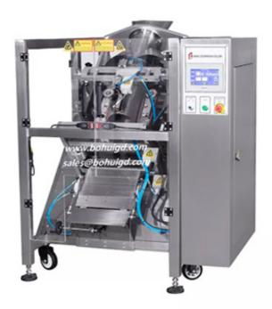
Dustial Machinery® BXD series inclined vertical packaging machine is mainly used for packaging fragile products such as biscuits, desserts, bakery products and other fragile materials in conjunction with weighing machines or dosing devices.
