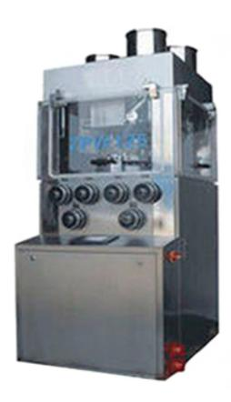
This machine is a single-press type, continuously automatic rotary tablet press for pressing various granular materials into tablets. It is mainly used in pharmaceutical industry of Chinese and western to produce large tablets, simultaneity adapted to chemical, food, and electronic industry.
