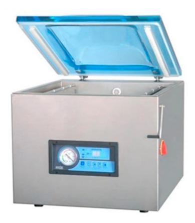
It is a commercial-grade vacuum packaging machine. It shares many characteristics with larger models, such as heavy duty oil-filled rotary vacuum pumps, sealing systems, and all-metal construction, but has a vacuum chamber designed for bags no wider than 10 inches.
