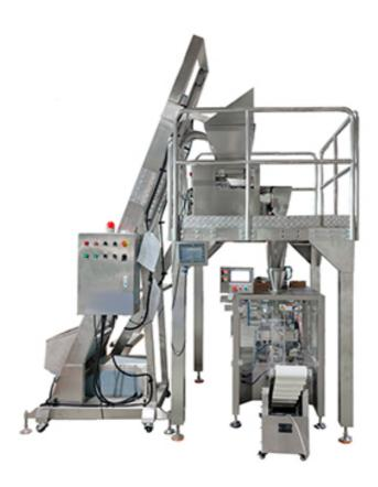
High Speed Multi-function Small Bag Packing Machine can link with multi-head weigher, powder srew conveyor, rotor pump or other many kinds of measuring machine to pack granule, powder or liquid in small bag. Speed can reach 150 bag/min, with 4 servo control.
