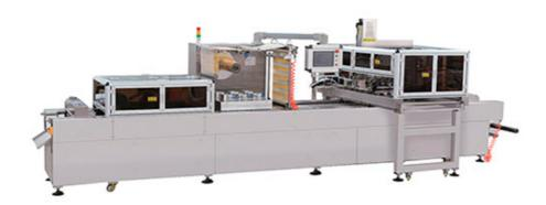
Full-automatic thermoforming and filling packaging line is special for various kind vacuum packed products, like pickled vegetable, meat product, grain products etc.
