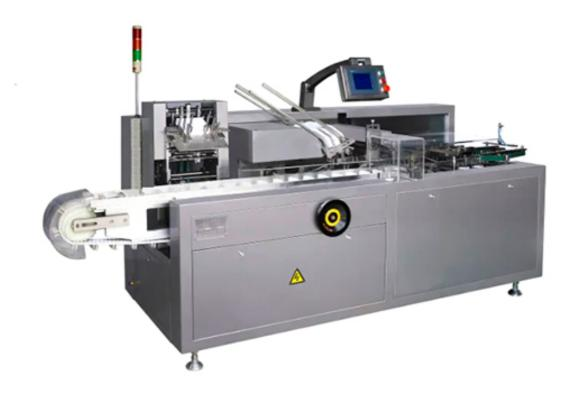
This machine is high technology product incorporates of pneumatic-photo-electro-mechanic. It is suitable for inserting bars, pillow wrapped products, pharmaceutical products and food similar package into carton in a range. The machine finishes running by a series of photo-electro controller to make the machine stability and guarantee the packing quality. It includes canton suction and open, products put into, printing batch number, sealing carton with tuck-in or hot melt glue device.
