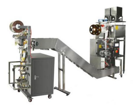
The MK-SJB02 vertical form fill seal machine consists of a tea bag former and outer envelope former for the packaging of tea bags and outer envelope. It carries out automatic feeding, weighing, bag forming, sealing, cutting, counting and finished package conveying, as well as outer envelope forming. The MK-SJB02 packaging machine is suitable for tea bag and outer envelope sealing of green tea, black tea, coffee, and more.
