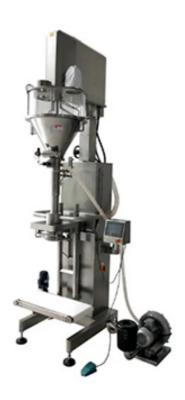
This model is designed mainly for the fine powder which easily to spout dust and high-accuracy packing requirement. Based on the feedback sign given by below weight sensor, this machine do measuring, two-filling, and up-down work, etc. It is specially suitable for filling additives, carbon powder, dry powder of fire extinguisher, and other fine powder which needs high packing accuracy.
