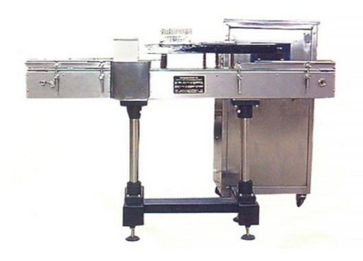
This machine is Applied to food, pharmaceutical, chemical, commodity industrial all kinds of vessel mouth aluminum foil sealing.
