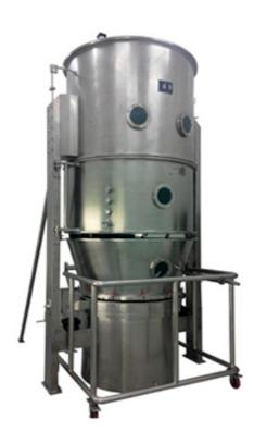
The method of boiling and granulating is a comprehensive fruit of spraying and fluidizing technology. It makes traditional mixing, granulating and drying processes finish in the same closed container. So it is called as "one step granulator".
