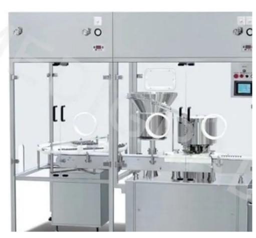
The capping machine continuously rolls the vials through a single, three or more capping knives. It can automatically complete the process of bottle feeding, top cover, rolling cover and bottle discharging. Equipment design and materials are fully compliant with cGMP regulations.
