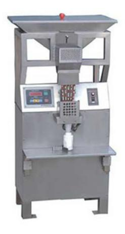
SSL-1 Semi-auto Capsule Counter is suitable for counting and filling the hard capsules into bottle. It is fixed with automatic counting device. Its operation and maintenance is simple. Counting speed can be adjusted by speed of loading bottles manually. The machine will stop counting automatically when one bottle is full, and start to count when empty bottle is loaded.
