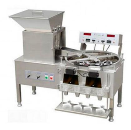
YL-4 Pill Counter Machine has been designed and developed to count & fill different shapes or size of products accurately like soft gel capsules, hard pill capsules, pill tablets, sugar coating, and film coating tablets, pills, herb medicine or similar products into containers or vials.
