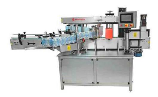
Double Side Sticker Labeling Machine: SVADL100/200/300 is fully automatic double side sticker labeling machine. This model has been designed to apply one, two or more front/back self adhesive labels on different size of flat/round/elliptical shape containers.
