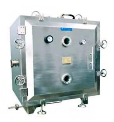
It is well known that vacuum drying is to put raw material under the state of vacuum for heating and drying. If use vacuum to pump air and humidity out, the dry speed will be faster. Note: if use condenser, the solvent in raw material can be recovered. If the solvent is water, condenser might be canceled and the investment and energy could be saved.
