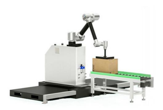
The workstation mainly includes a handling robot, a mechanical grasp, and two sets of product-blocking devices, a safety bar, and a control system
