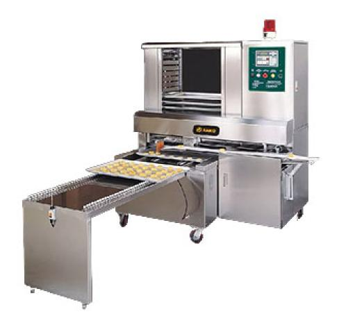
The microcomputer-controlled Automatic Aligning Machine allows users to store 9 sets of parameters for different arrangements. With automatic tray placement, it helps you save labor costs and improve efficiency. The Aligning Machine features high flexibility in working with Encrusting and Forming Machine as well as Stamping Machine to deliver fully automatic production. This production line can produce 2,400 pieces per hour, satisfying the requirements of both stable quality and high capacity.
